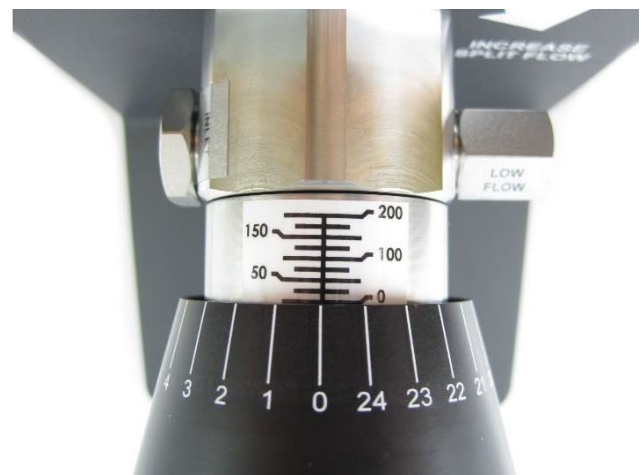
Figure 4: Split flow Vernier scale on splitter body
